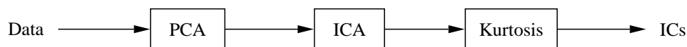
Figure 1: The proposed ICA procedure. First, the data set is reduced by PCA thereby maintaining all of the relevant variances. ICA is applied to this reduced data set and the extracted independent components are sorted by their kurtosis value.
